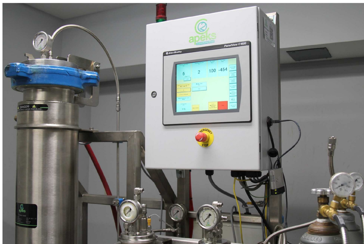
Figure 4. Supercritical extraction instrument for cannabis oil production.
